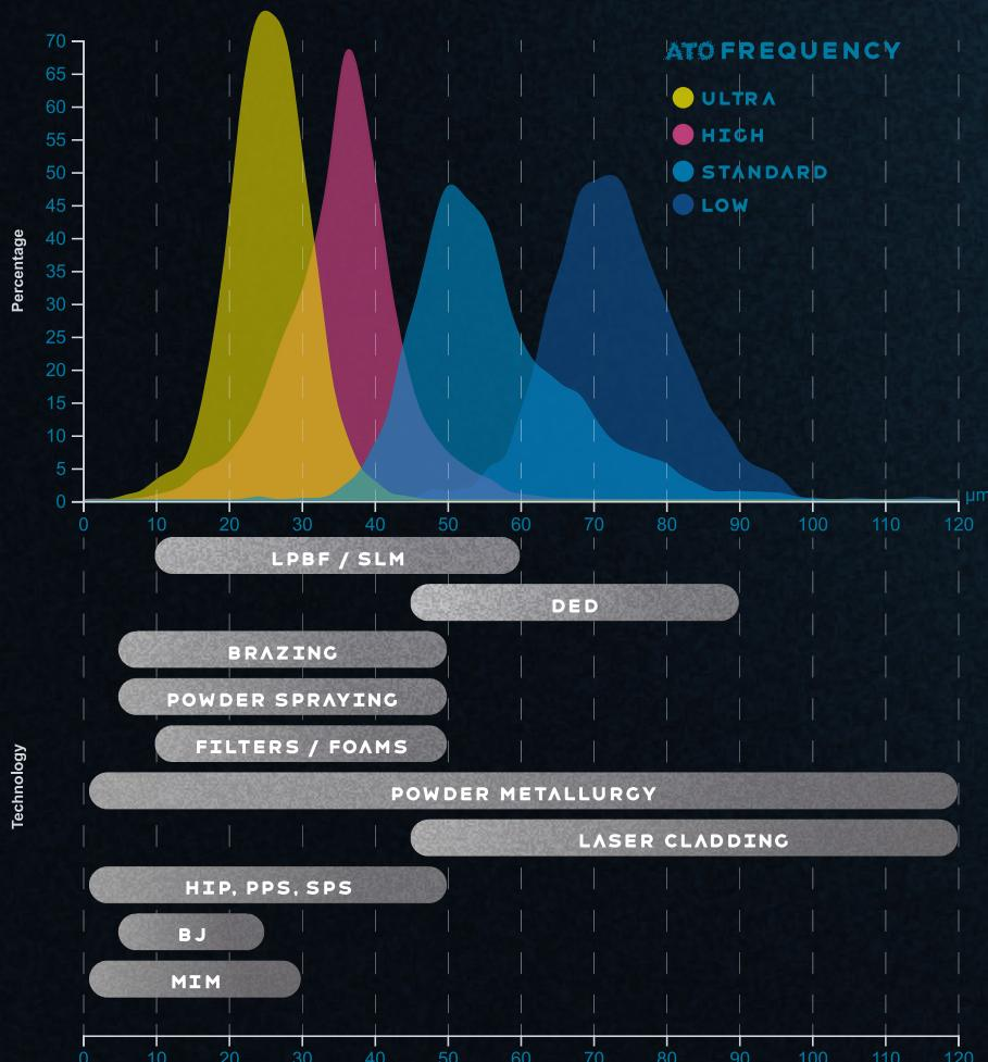
\* The diagrams show actual atomization results of 316L stainless steel using various ultrasonic frequency systems. Results may vary based on feed materials, properties, spray parameters, process conditions and other variables.
