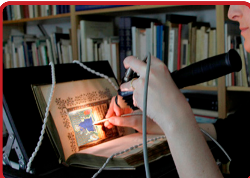
A FieldSpec 4 instrument being used to characterise both organic and inorganic materials in pigments and binders on a number of illuminated manuscripts.
