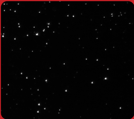
The 10x objective of the ZetaView allows analysis of up to 200 particles in the field of view – yielding superior concentration results.
