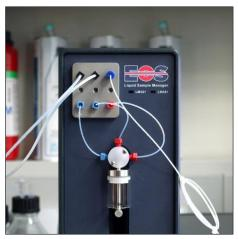
Quartz, BK7, PTFE, PCTFE, FEP, FFKM, PEEK, and Stainless Steel wetted surfaces ensure high chemical compatibility. CLASSIZER™ ONE measures samples at laminar constant flows of 0.2, 0.5, 1.0, 2.0, 4.0 mL/min and viscosity up to 10cS.
