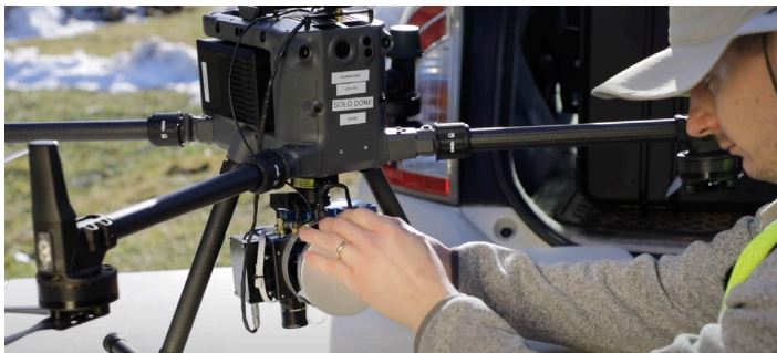
Figure 1. Headwall UAV systems utilize a quick-release mechanism between the drone and the payload that allows easy removal of the sensor suite for transportation or storage.
