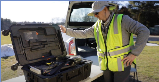
Some UAVs such as the DJI Matrice 350 can be folded into a more compact shape for transport to and from your mission location.
