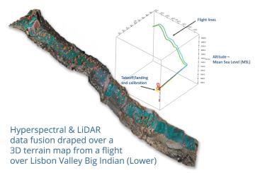
**Figure 3.** A single flight over challenging terrain captured both hyperspectral data over the VNIR to SWIR (400–2,500nm) wavelength range and a high-resolution LiDAR point cloud, enabling this exquisitely detailed orthorectified and geo-located 3D image.
