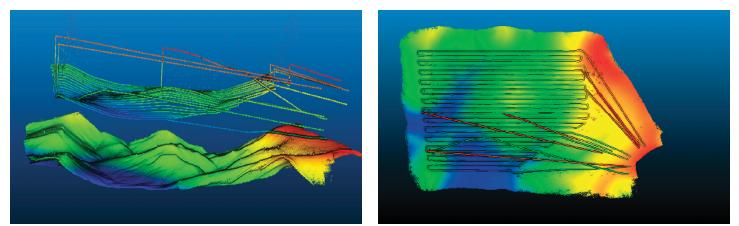
**Figure 4.** The images above are 3D point clouds generated from an optional LiDAR sensor that was part of the payload during a hyperspectral UAV mission to Cuprite, Nevada by a team from Headwall and the University of Arizona. LiDAR allows high-resolution digital elevation models (DEMs) to be created to enable more precise flight operations as well as more accurate orthorectification of the hyperspectral imaging data.
