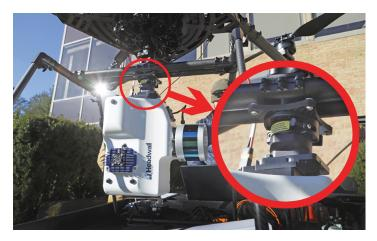
**Figure 1.** Headwall UAV systems utilize a quick-release mechanism between the drone platform and the payload that allows easy removal of the sensor suite for transportation or storage.
