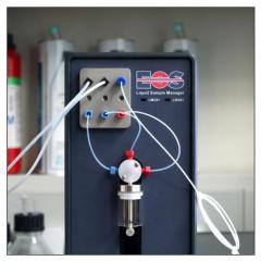
Quartz, Borosilicate Glass, PTFE, FEP, FFKM, FKM, and Stainless Steel wetted surfaces ensure high chemical compatibility. CLASSIZER™ ONE measures samples at laminar constant flows of 0.2, 0.5, 1.0, 2.0, 4.0 mL/min and viscosity up to 30cS.
