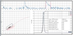
Online/InLine monitoring of particles during continuous flow processes lasting hours or for measuring samples injected using an external commercial autosampler. CLASSIZER<sup>TM</sup> ONE may start/stop acquisitions via an external communication protocols as RS485, square volt, or tailored com protocols developed to fit user needs.
