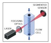
How CLASSIZER<sup>TM</sup> ONE / SPES works. A sample is dispersed and diluted in a liquid, which is flowed through a scattering cell where a laser beam is properly shaped and focused. As a single particle crosses the laser beam, the interference pattern between the transmitted beam and the forward scattered light is recorded on a sensor. The interference pattern presents fringes delivering the unique optical properties of the single particle illuminated.
