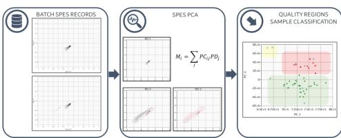
Supervised Machine Learning and K-nearest neighbour method available to classify batches using discrete labels as True/False, Yes/No, OK/Not OK, or Good/Bad to evaluate new data against library of previously measured batches.
