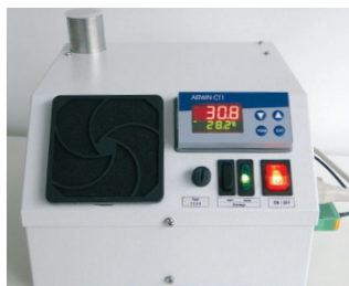
Ultrasonic humidifier to prevent evaporation and for dew point pipetting
