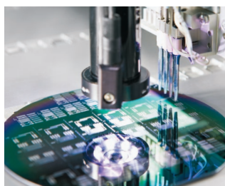
Microscope for optical target recognition / spot adjustment
