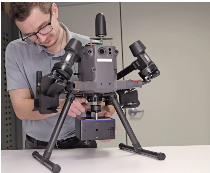
Figure 1. Headwall UAV systems utilize a quick-release mechanism between the drone platform and the payload that allows easy removal of the sensor suite for transportation or storage. Some systems may be configured for use on a Field Rotary Kit to gather ground-truth data in the field.
