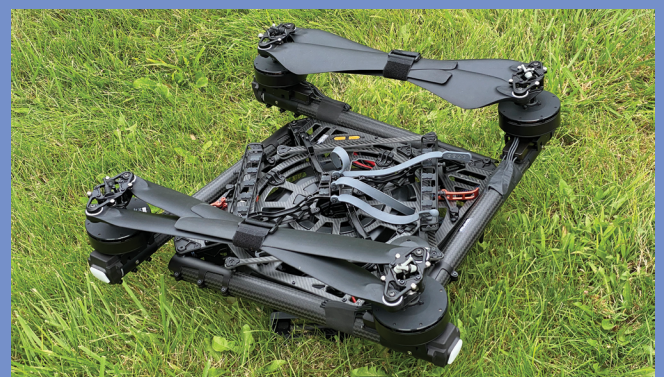
The FreeFly Alta X UAV can be folded into a more compact shape for transport to and from your mission location.
