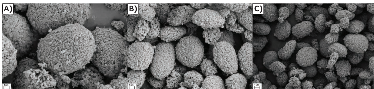
Figure 3. SEM images of \text{Ni}_{0.8}\text{Co}_{0.1}\text{Mn}_{0.1}(\text{OH})_2 precursor materials synthesized via the CTFR (pH value: 12; T : 60 °C; \tau : 4 h) showing the dependence of the rotational speed ( \omega_i ) of the inner cylinder. A) \omega_i : 500 rpm; B) \omega_i : 900 rpm; C) \omega_i : 1300 rpm.
