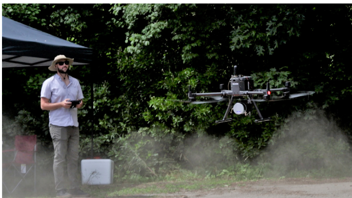
Figure 4. Customer Success Engineer and FAA-Certified Drone Pilot Charles Kepler flying the drone holding the Nano-Hyperspec VNIR sensor
