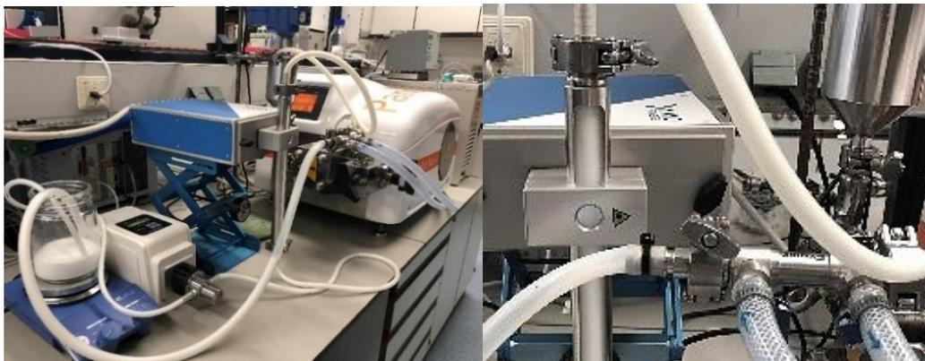
**Figure 6** Set up for inline monitoring of the droplet size using the NFS during homogenization of the O/W emulsions.
