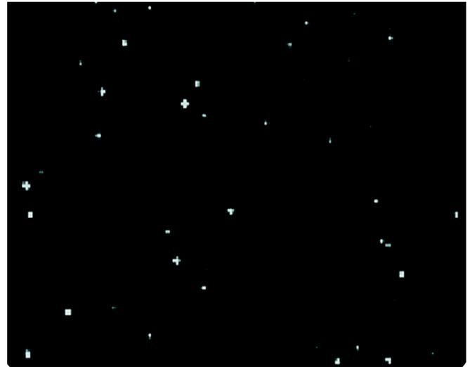
The 10x objective of the ZetaView allows analysis of up to 600 particles in the field of view – yielding superior concentration results.
