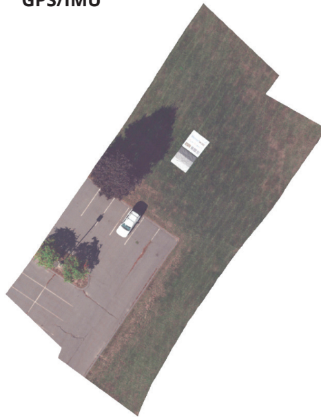
Figure 3. Ortho-mosaicking using the Standard (Gen 2) GPS/IMU can be visually comparable to the High-Performance GPS/IMU. So, why use the High-Performance GPS/IMU? The vertical accuracy of the High-Performance GPS/IMU is significantly better than that of either model of the Standard (Gen 1 or Gen 2) GPS/IMU. This can be crucial for applications that require accurate LiDAR point-cloud data. See the Geolocation Error table and the Specifications table below.
