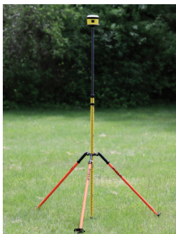
Figure 4. Headwall offers an optional Smart Target Base Station that compares its own fixed location to generate GPS error-versus-time data to correct drone GPS measurements.
