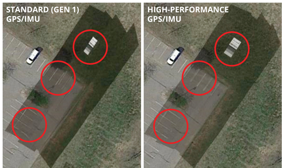
Figure 2. Multiple flight swaths were orthorectified and stitched together in the above images, left using the Standard (Gen 1) GPS/IMU and right using the High-Performance GPS/IMU. Notice the image distortions of the parking lot lines and the reflectance tarp with standard GPS/IMU data. The legacy Standard (Gen 1) GPS/IMU system had a single GPS antenna, and at speeds below 10 meters per second, the resulting ortho-mosaicked images can be inferior to those produced using the High-Performance GPS/IMU.
