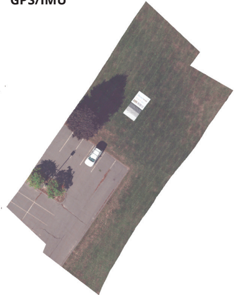
Figure 3. Ortho-mosaicking using the Standard (Gen 2) GPS/IMU can be visually comparable to the High-Performance GPS/IMU. So, why use the High-Performance GPS/IMU? The vertical accuracy of the High-Performance GPS/IMU is significantly better than that of either model of the Standard (Gen 1 or Gen 2) GPS/IMU. This can be crucial for applications that require accurate LiDAR point-cloud data. See the Geolocation Error table and the Specifications table below.
