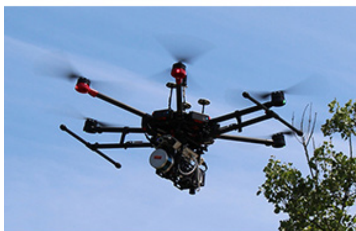
Headwall's integrated airborne solutions combine high-precision GPS/IMU instruments as well as LiDAR
