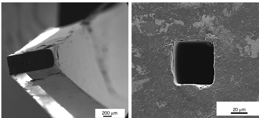
**Figure 1:** SEM-image of the inkjet nozzle (Nano-Tip-J-H, A070-570, GeSiM): Overview image of the whole inkjet nozzle (left) and detailed image of the cubic pinhole (right).
