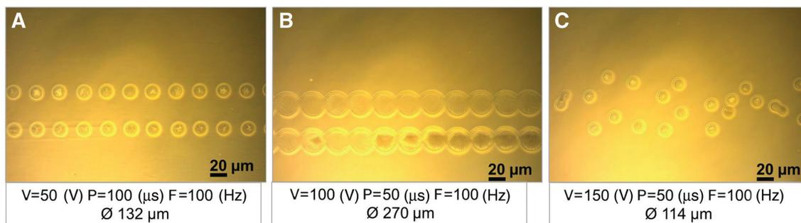
**Figure 3:** Light microscopic images of the size of spots generated by the adjustment of different parameter.
