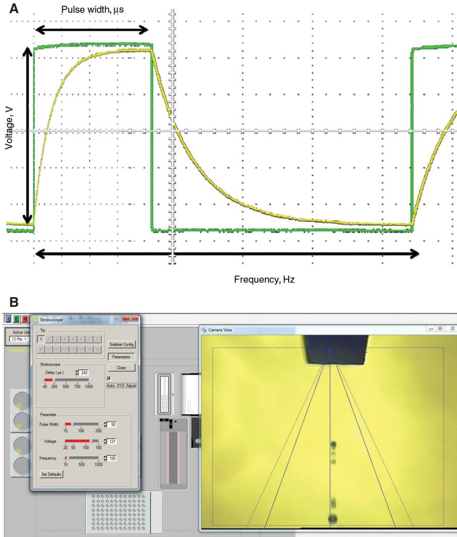
**Figure 2:** (A) Voltage – frequency plot to illustrate the correlation of the piezo printing parameter voltage (V), pulse width ( $\mu\text{s}$ ), frequency (Hz). (B) The control interface of the inkjet printer showing the analysis of the droplets with angle failure (image from the stroboscope camera of the BioScaffolder). This allows observing the droplet formation after the inkjetting.
