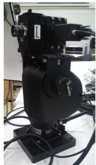
Figure 1- Hyperspectral instrument - Headwall Photonics, Inc. Hyperspec A-series placed on Pan&Tilt mobile unit
