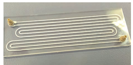
Examples of additive manufacturing. Top row: polycaprolactone (PCL) cylinders, melt electrospraying of PCL and printed microfluidic channels. Bottom row: alginate scaffold and scanning electron micrograph of a bone cement scaffold after setting (material: InnoTERE, Radebeul).
