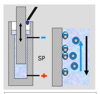
**Stabino® principle:** Piston moving up and down in the measurement cylinder, inducing the particle interface potential SP and mixing during auto-titration.
