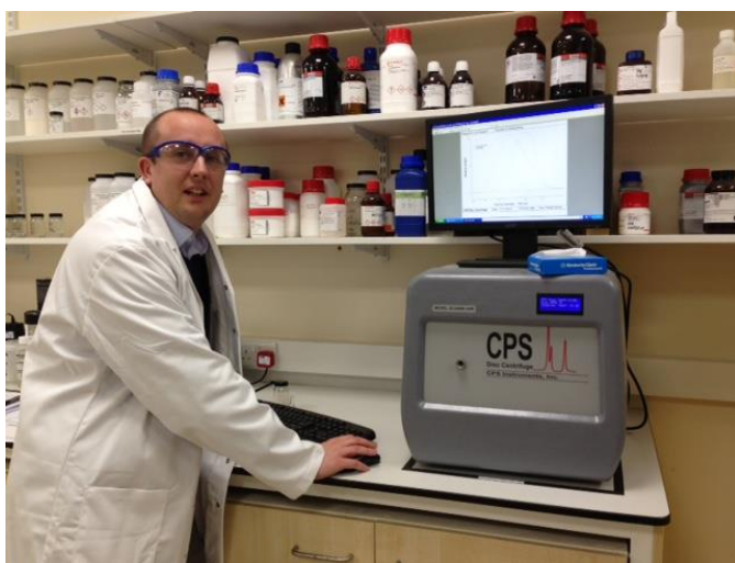
Luke Alger, Scott Bader's polymer development manager, using the CPS Disc Centrifuge for measuring conventional and inverse emulsions
