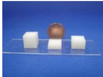
Cubes of PCL at a molecular weight of 14,000. The cubes have X, Y dimensions of 10 mm by 10 mm. The heights of these examples are 10 mm, 3 mm and 7 mm (Left to right).
