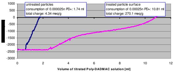
The untreated sample (blue) consumes much less calibrated cationic Poly-DADMAC than the modified one (red). The density of COOH charge at the treated CNT interface was 270 meq/g sample.
