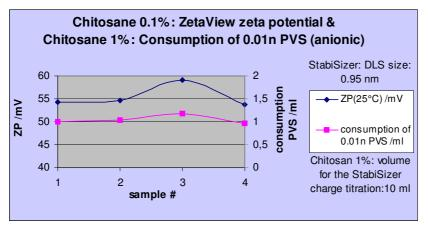
Although the lower size limit of ZetaView® is at 80 nm size. the measurement on a few Chitosan agglomerates deliver could very reasonable zeta potential results. The correlation of the StabiSizer® polyelectrolyte consumption (titration curves below)
