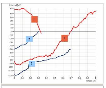
1a-Red: Titration with cationic polymer solution, followed by 1b-Red: titration with anionic particle suspension
